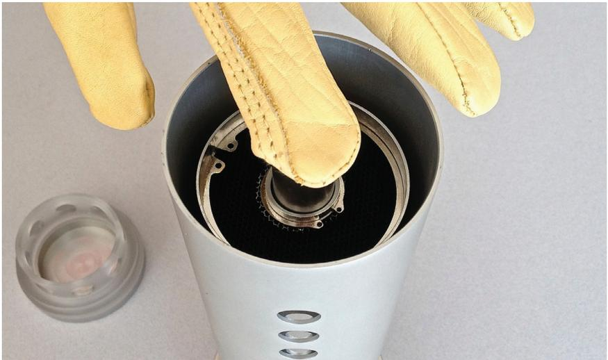
6. You are now ready to reassemble the unit. Insert the top cap into the aluminum body so that the screw holes in the aluminum line up with the threaded holes in the top cap. Reinsert the screws and plug in the power supply. If your air purifier functions normally again, your lamp replacement has been successful.
