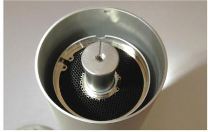
3. Remove the top cap. This will give you a clear view into the top of the air purifier. The photo on the right shows the UV chamber with the UV lamp inserted in its center. Note that the UV chamber has a half-round notch in its wall and that the lamp end cap has a groove in its top. The notch and the groove will be in alignment.
